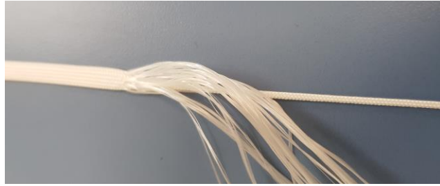
Diameter change from 48 to 16 carriers
